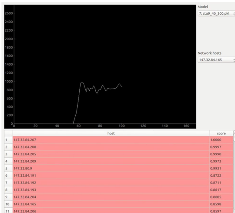
Figure 4.3.8. A window from a later stage of the infection, where the botnet has been active for some time and botnet traffic is at a peak. All infected hosts are identified as active bots.
